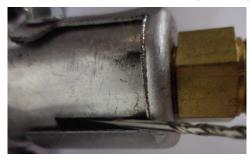
Figure 4 (Measure opening using drill bit)
