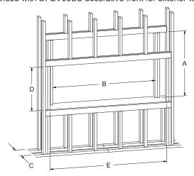
Figure 14 - Rough Opening for Elevated Installation
