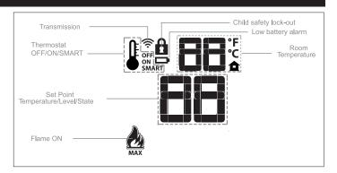
Figure 72 - Transmitter LCD display
