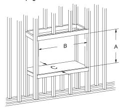
Figure 13 - Rough Opening for Elevated Installation
