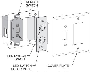
Figure 73 - Proflame Receiver Body Front
