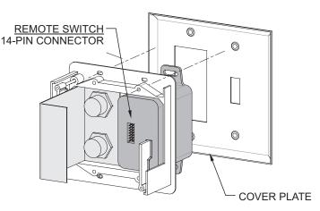
Figure 74 - Proflame Receiver Body Back
