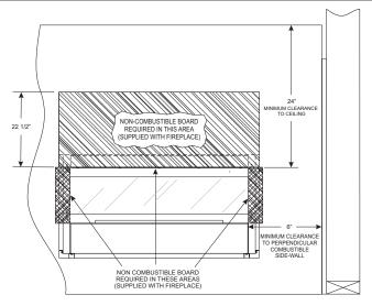
**NOTICE:** Combustible material is allowed below a fireplace viewing area opening and outside the non-combustible board.
