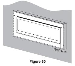
3b. Exterior non-combustible finishing material is placed over the face of the outdoor kit. **See Figure 61.**
